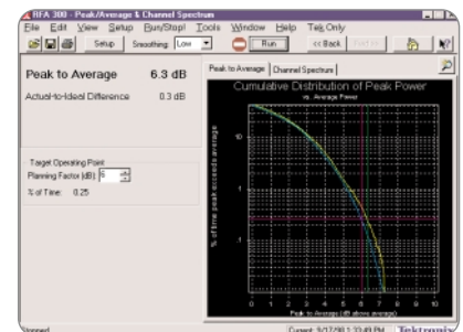
► Peak to Average Power and Actual-to-Ideal Difference with Cumulative Distribution of Peak Power and Channel Spectrum Graphics.
