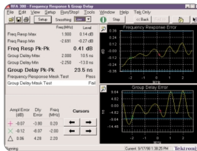
► Frequency Response and Group Delay Measurements with Graphical Displays of Errors.
